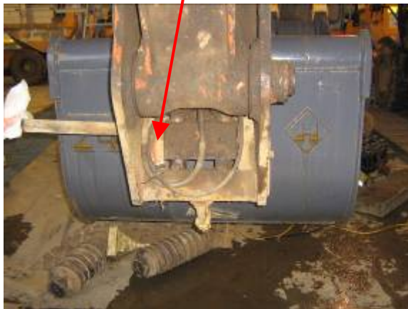
Photo 3. Best practice – Welded lug on end of safety bar prevents full withdrawal
