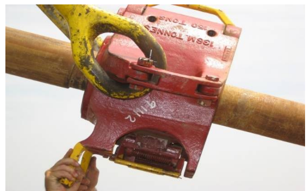
Casing elevators clamped onto a drill collar
